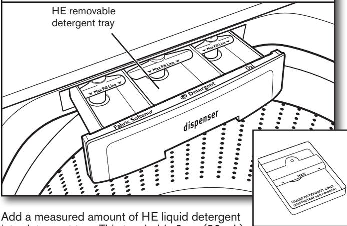
Add a measured amount of HE liquid detergent into detergent tray. This tray holds 3 oz. (89 mL). If adding powder HE detergent remove inside tray. Do not overfill tray – adding too much detergent may cause detergent to be dispensed into the washer too early.
