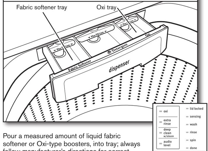
Pour a measured amount of liquid fabric softener or Oxi-type boosters, into tray; always follow manufacturer’s directions for correct amount of fabric softener or Oxi based on your load size.
